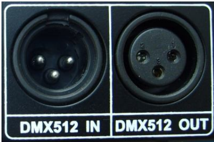
3-pin-block as DMX signal interface.
